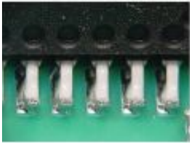
Figure 5B. QFN soldered with rosin.
