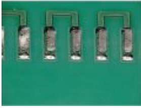
Figure 5A. QFN soldered with water-soluble paste.
