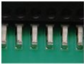
Figure 5C. QFN soldered with no-clean.
